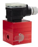
The flow meter measures the moving dosing volume of liquids according to the gearwheel principle. A pair of gears fitted very precisely into the housing forms the measuring mechanism. The rotation of the measuring mechanism is detected tooth by tooth without contact by a signal pickup system and converted into digital pulses.
